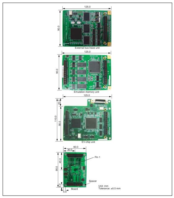
Figure 7 Dimensions for External Bus Trace Unit, Emulation Memory Unit, EV-Chip Unit, and User System Interface Board
